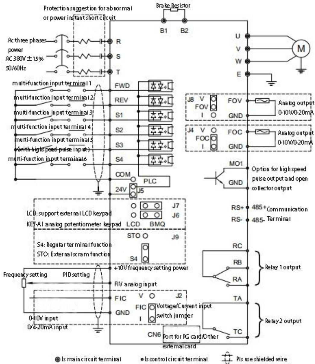
Note: It is built-in braking unit for below 37kW, the braking unit is optional for 45-160kW
